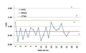
Coefficient of variation (CV%) of DHI mixed pigments injected three times for each data set. Three instances (red squares) where the CV% increased were identified. A fault in the HPLC auto-injector was corrected and the CV% was restored.
