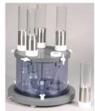
The filters are held by chimneys made of acid-resistant stainless steel, with a capacity of either 20 mL or 100 mL. The base of each chimney is composed of Teflon (PTFE) and stainless steel. Additionally, by placing the chimneys in a freezer, chilled filtration (e.g., TCA) can be carried out. The top and bottom of the manifold and the cylinder collecting filtrates are made of PVC.
